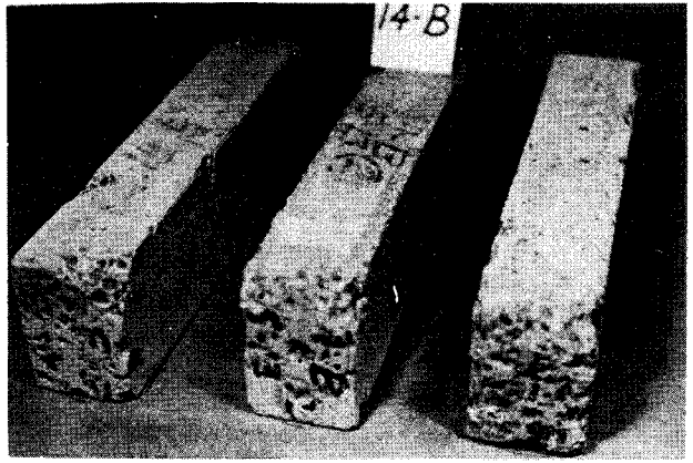
Mix No. 14-B - 502 Cycles of Freezing and Thawing
