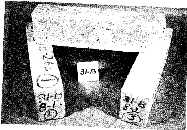
Mix No. 31-B - 83 Cycles of Freezing and Thawing
