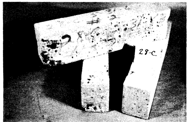
Mix No. 28-C - 502 Cycles of Freezing and Thawing
