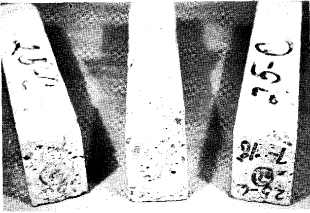
Mix No. 25-C - 501 Cycles of Freezing and Thawing
