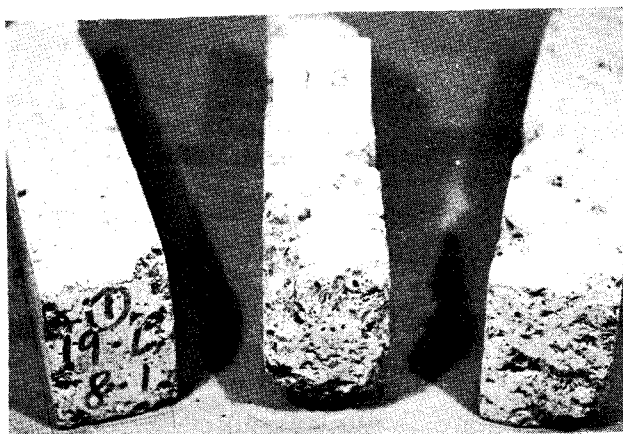
Mix No. 19-B - 463 Cycles of Freezing and Thawing
