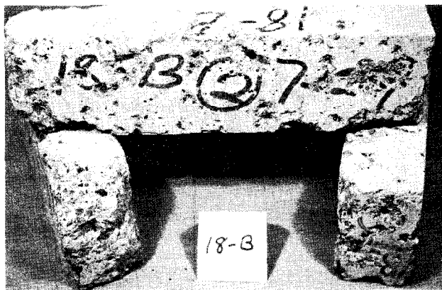
Mix No. 18-B - 494 Cycles of Freezing and Thawing
