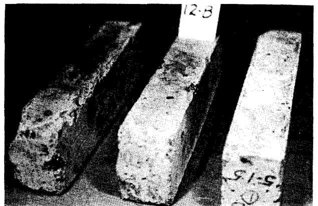
Mix No. 12-B - 504 Cycles of Freezing and Thawing
