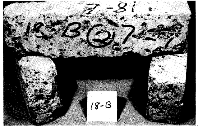
Mix No. 18-B - 494 Cycles of Freezing and Thawing
