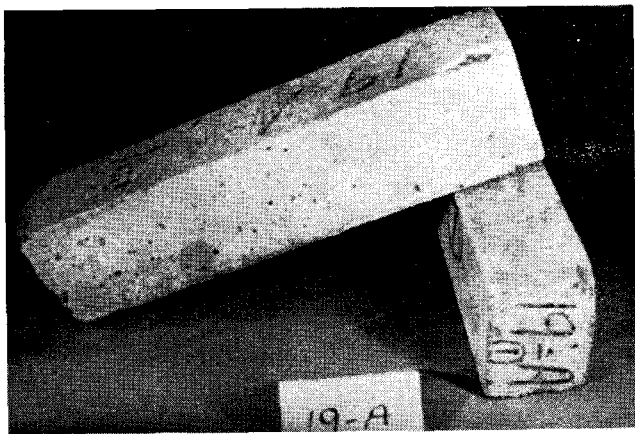
Mix No. 19 - A - 300 Cycles of Wetting and Drying
