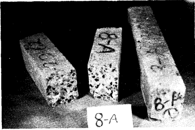
Mix No. 8 - A - 300 Cycles of Wetting and Drying
