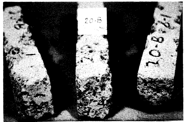
Mix No. 20-B - 466 Cycles of Freezing and Thawing
