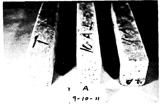
Mix No. 9 - A, 10 - A, and 11 - A - 300 Cycles of Wetting and Drying
