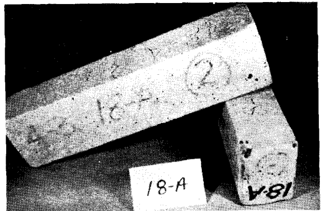
Mix No. 18 - A - 300 Cycles of Wetting and Drying
