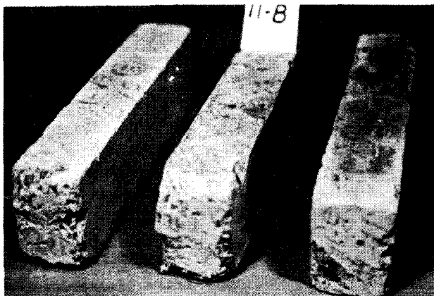
Mix No. 11-B - 504 Cycles of Freezing and Thawing
