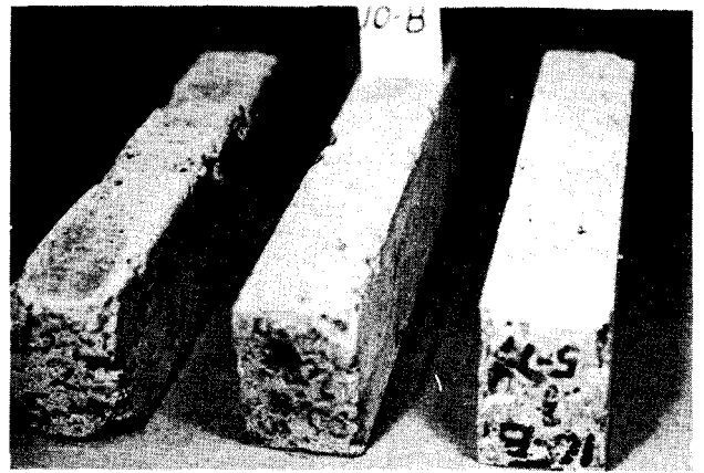
Mix No. 10-B - 504 Cycles of Freezing and Thawing
